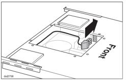
■ Plug the connector for the blower into the socket in the housing as shown.
